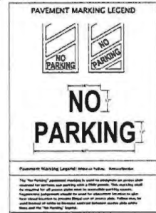
3 NO PARKING PAVEMENT MARKING 1/2" = 1'-0"
