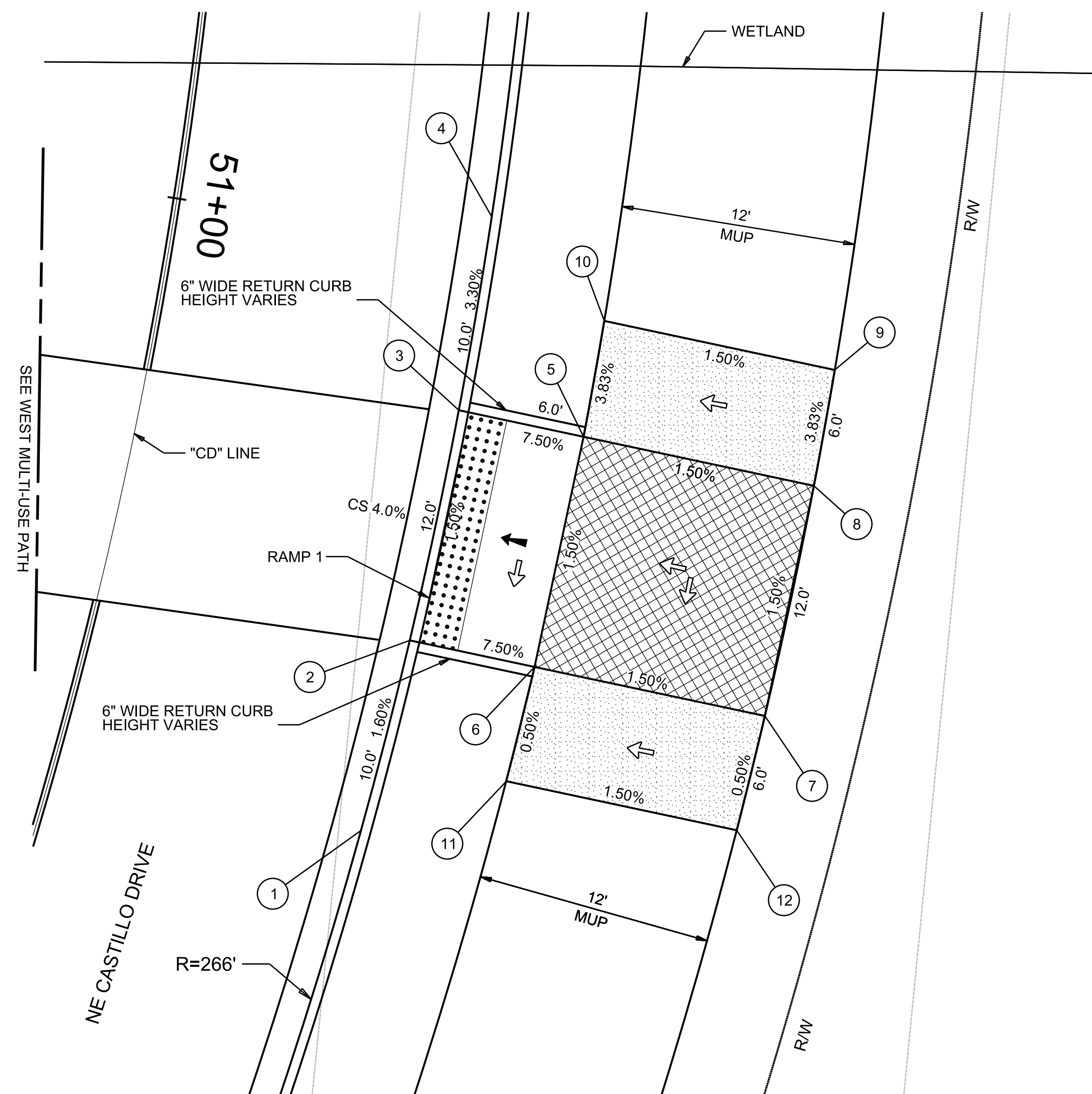
EAST MULTI-USE PATH CROSSING NE CASTILLO DRIVE EXTENSION
